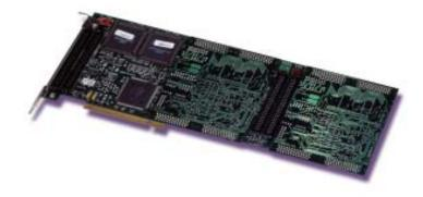
The CEI-500 is a flexible, space-saving, multi-protocol solution for the PCI platform. Based on rugged and versatile IP module technology (also known as IndustryPack), the CEI-500 provides the proven advantages of open system design while supplying a large number, of low cost ARINC 429, CSDB, RS-232, RS-422, RS-485, MIL-STD-1553 and other interfaces on a single board
