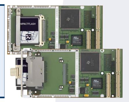
PMCF3 is a member of Radstone's extensive family of COTS IEEE 1386.1 compliant PMCs (PCI Mezzanine Cards), offering a convenient way to add large capacity, non-volatile memory to rugged system solutions. Targeted at the world's defense and aerospace OEM marketplace, this cost effective CompactFlash adapter is ideal for use with Radstone's families of COTS SBCs and PMC carrier cards. PMCF3 can be plugged on to any host with a PMC site \* and is available in five ruggedization levels.
