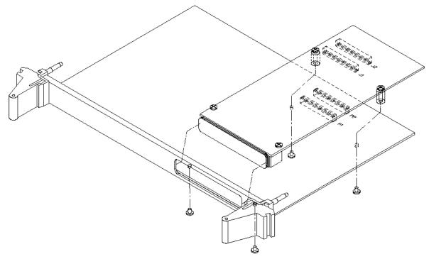
Use screws to fasten PMC card to the host CMC.
