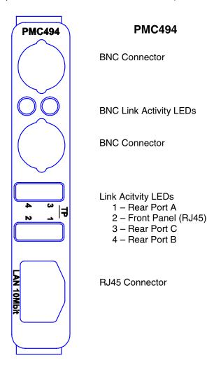
• The two BNC connectors of the PMC494 facilitate connection in the middle of the coax segment without need of using a BNC "T."
