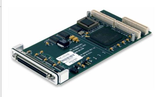
**PMC-USCSI320** provides a single channel high-performance ULTRA320 SCSI adapter for a PMC carrier board in VME, CompactPCI, or PCI-based systems. It is ideal for disk, tape, CD-ROM or other storage media and SCSI peripheral applications. The cards supports single-ended or differential signaling for asynchronous or synchronous SCSI operations. Flexible physical I/O access is available via a 68-pin SCSI-III front-panel connector.
