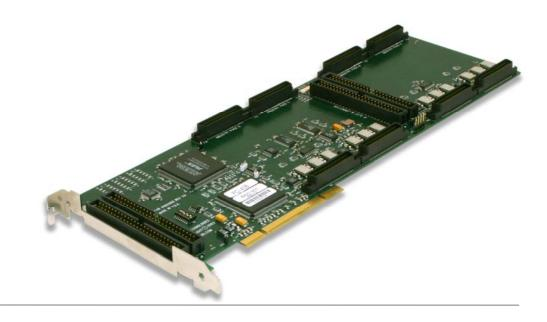
PCI-40B is an IndustryPack® carrier board that provides four IndustryPack slots on a single desktop or industrial PCI slot card. The IndustryPack bus clock is software selectable on a per-slot basis between 8 and 32 MHz.
