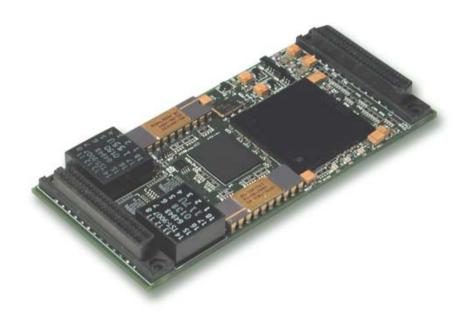
The Condor Engineering IP-D1553 takes MIL-STD-1553A/B technology to a new level on a single-wide IP Module. It is available in commercial or extended temperature configurations with either one or two dual-redundant, single or multi-function interfacees.
