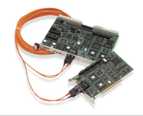
**SBS bus-to-bus adapters** directly connect two buses. The virtual bus created allows the two systems to operate as one, enabling seamless operation, superior performance, and if the two buses are dissimilar, such as a PCI bus and a VMEbus, the combined benefits of two diverse systems.
