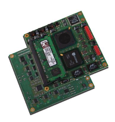
**XCOM-9347** is a highly integrated solution specially designed to meet PICMG COM.0 standard requirements. It features a low-power high-performance PowerPC processor in COM Express Compact (microETXexpress) form factor, only 95x95 mm
