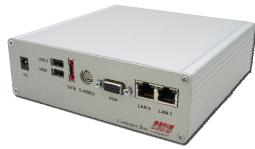
XBOX-9347 is a highly integrated computer box solution, measuring 165x160x52 mm (6.5x6.2x2 in), based on the PICMG COM Express processor module standard. It features a complete computer system with its complete set of peripheral I/Os ready to use for embedded applications.
