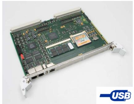
VSBC-6848 VME PowerQUICC II Single Board Computer are based on the MPC8248 processor. This processor is rated at 760 DMIPS @ 400 MHz.
