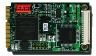
**MADC-1816** offers simultaneously sampling A/D architecture with 8 single-ended or 4 differential analog input channels. All channel features programmable gain 1 or 2 and can program to handle analog input with a single-ended or differential configuration.
