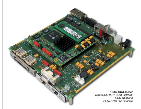
KCAC-0320 is a highly integrated solution, measuring 160x160mm (6.3x6.3 in), specially designed to meet COM Express PICMG COM.0 standard requirements. It features a complete COM Express carrier solution for processor modules sized in Compact (95x95 mm) and Basic (125x95 mm) form factors.
