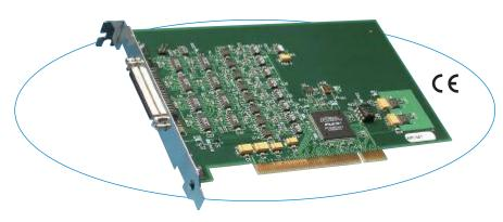
This board is ideal for high-speed data acquisition. A large memory buffer reduces CPU interactions for increased overall performance.
