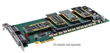
Four AcroPack or mini-PCle mezzanine module slots ◆ Non-Intelligent carrier ◆ 3/4-length PCle x4 interface
