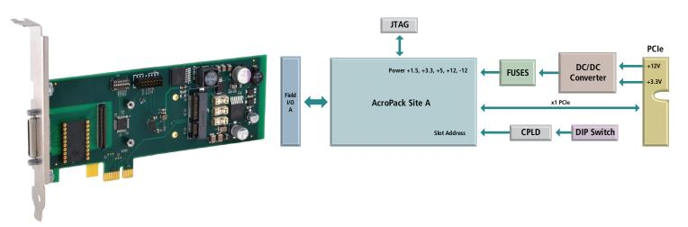
One AcroPack or mini-PCIe mezzanine module slot ◆ Non-Intelligent carrier card ◆ PCIe x4 interface
