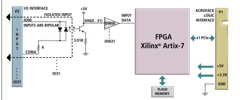
32 Isolated Digital Input Channels • Extended Temperature
