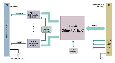
16-bit DAC ◆ 16 Channels Voltage Output ◆ Wide Temperature Range ◆ PCIe Bus Interface
