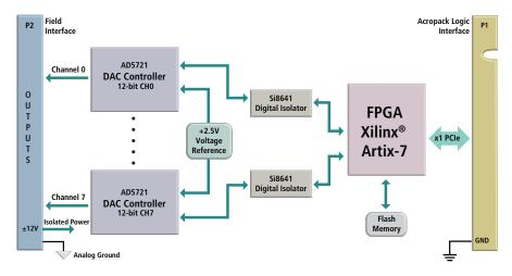
12-bit DAC ◆ 8 Channels Voltage Output ◆ Wide Temperature Range ◆ PCIe Bus Interface
