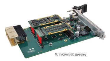
3U CompactPCI Serial ◆ Two I/O expansion slots (AcroPack or mPCIe) ◆ Rear I/O access
