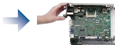
2. Insert the optional fan module by gently slide it into the fan connector
