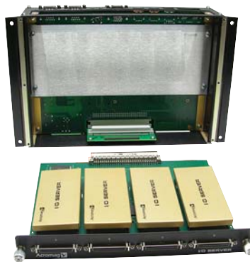
Above: A bottom view shows the heat spreader plate that removes heat from the I/O modules.
