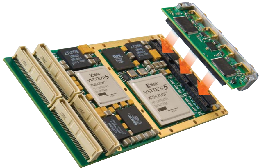
AXM-A30 Analog I/O plug-in extension module.
